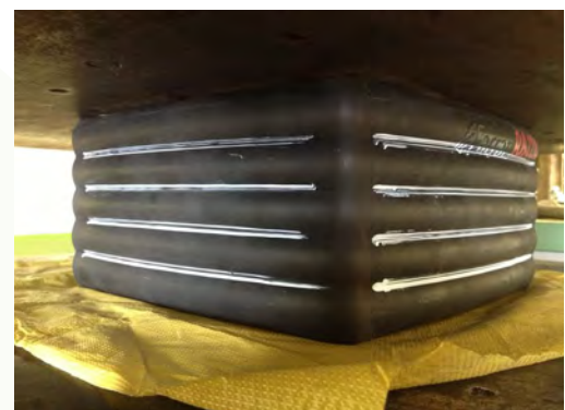
Fig 8.2 Five-Layer LNR Bearing Under Compression Load
