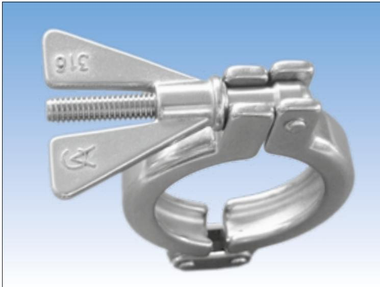
The 'gate' style section combined with the stepped eyebolt ensures that the clamps bolting mechanism cannot swing open whilst the clamping union is partly or fully assembled.
