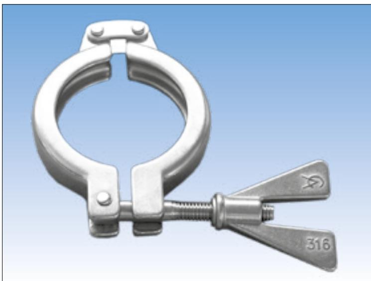
Releasing the clamp is only possible when the wing nut has been significantly loosened to enable the smaller diameter of the eyebolt to swing open and pass through the sectioned gate; this ensures the clamp cannot be knocked or accidentally opened. Complete wing nut removal is not necessary to open the clamp but the design guarantees that the eyebolt cannot swing open whilst the union is subjected to either clamping forces or internal pressure.
