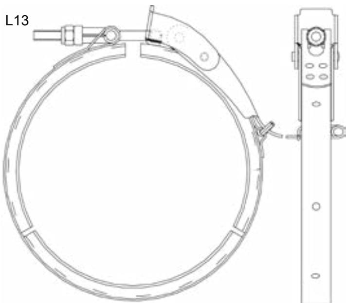
One T-Bolt with Toggle Lever Safety Pin
