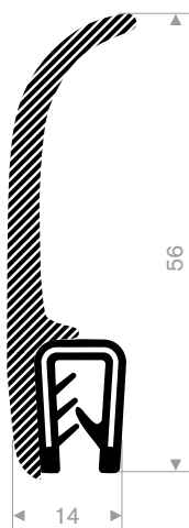
pvc + Sponge rubber clamping range 1-3 mm roll length 25 meter
