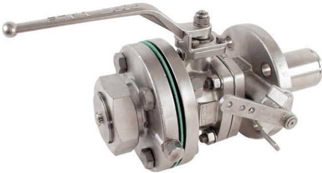
2" Short Profile Footvalve for compressed liquefied gas - 500 PSI (34.5 Bar) pressure setting. Inlet flange drilled 4 x 18mm holes equi-spaced on a 125mm PCD. DIN 50 PN 40. Complete with 2" ball valve. Left hand operation. Contact parts manufactured in 316 stainless steel. Supplied with a 3.25" ACME outlet and cap.
