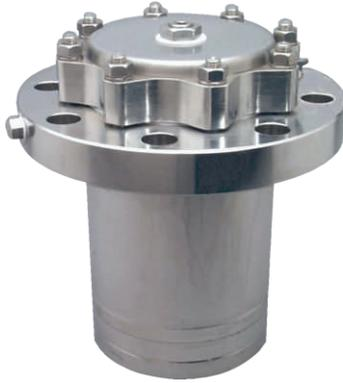
MKII 80mm Internal Gas Relief Valve & Bursting Disc Holder- Suitable for a pressure range of between 100 - 505 PSI (6.90 - 34.82 bar). Contact parts manufactured in 304/316 stainless steel. Fitted with PTFE seals as standard.
