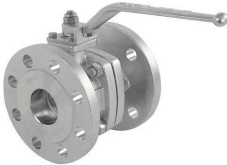
**2" Full Bore Gas Ball Valve** - DN 50 PN 40 high pressure valve. Flange drilling: 4 x 18mm holes on a 127mm PCD (2" ASA150) and 8 x 18mm holes on a 127mm PCD (2" ASA 300). Right hand operation. Contact parts manufactured in 316 stainless steel with PTFE seals.
