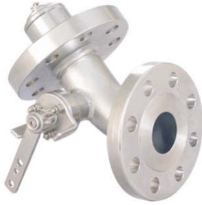
2" Liquid Phase Excess Flow Gas Footvalve - with 70° actuator. 500 PSI (34.5 Bar) pressure rating. Inlet flange drilled 8 x 18mm holes on a 127mm PCD. 2" ASA 300lbs. Contact parts manufactured in 316 stainless steel.
