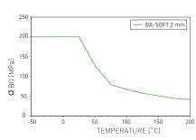
**P-T diagram** indicates the maximum permissible combination of internal pressure and service temperature which can be simultaneously applied for a given gasket's thickness, size and tightness class. Given the wide variety of gasket applications and service conditions, these values should only be regarded as a guidance for the proper gasket assembly. In general, thinner gaskets exhibit better P-T properties.
