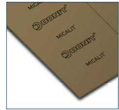
MICALIT<sup>®</sup> P contains a high percentage of phlogopite mica flakes, impregnated with a silicone binder and reinforced by a tanged stainless steel insert. It has excellent thermal, good chemical and mechanical properties, making it suitable for high temperature and pressure applications in the automotive and steel industry for exhaust systems, gas turbines, oil and gas burners, furnaces and ovens. It also offers good dielectric and low thermal conductivity properties.
