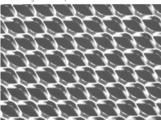
Composition: expanded natural graphite with >98% graphite purity (> 99% initial purity) laminated by a special process to an expanded chromium-nickel-steel insert (AISI 316L- 0.15 mm).
